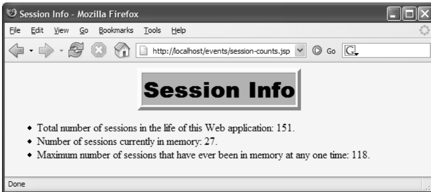
Figure 6-11 The SessionCounter listener keeps track of the sessions used in the Web application.
