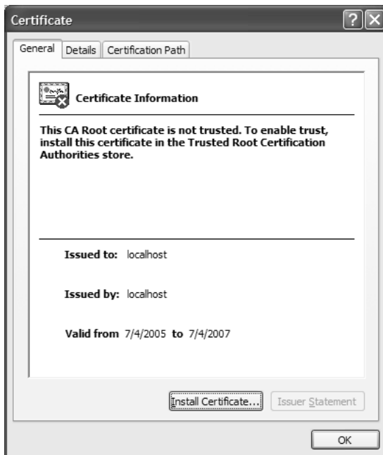
Figure 3–24 Certificate information presented by Internet Explorer. View different types of certificate information by clicking the General, Details, and Certification Path tabs at the top of this dialog box. To suppress future warnings, you can import the certificate by clicking the Install Certificate button and starting the Certificate Import Wizard shown in Figure 3–25.
