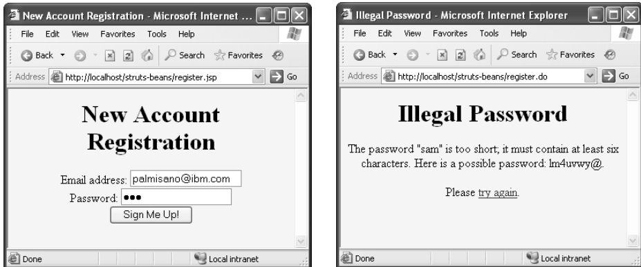
Figure 10–16 Registration form with an illegal password—one that doesn't contain six characters (left). Response for a "bad-password" condition (right). The bean:write tag displays both the bad password (from the form bean) and suggested password (from the suggestion bean).
