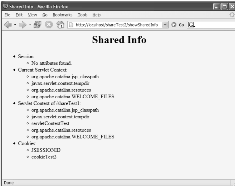
Figure 1–10 Result of visiting the SetSharedInfo servlet in one Web application and the ShowSharedInfo servlet in a different Web application.
