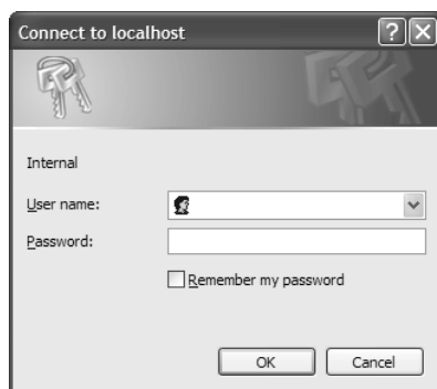
Figure 5–11 If the SecurityHolePlugFilter is enabled, it converts the RequestDispatcher.forward call into a direct client request. This invocation becomes no different than trying to directly invoke http://localhost/filtersrus/secure/job-openings.html , therefore the server asks for username and password to proceed.
