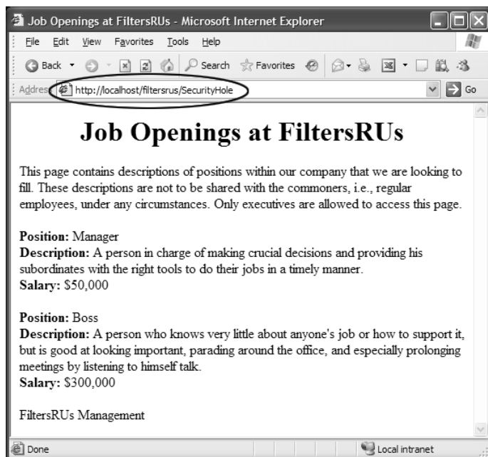
Figure 5–10 If the SecurityHolePlugFilter is disabled, the SecurityHoleServlet is able to bypass the security constraint and access the protected resource (i.e., /secure/job-openings.html ) without being authorized to do so. Because we are using the RequestDispatcher.forward method, the originally requested URL is showing in the browser's address bar.
