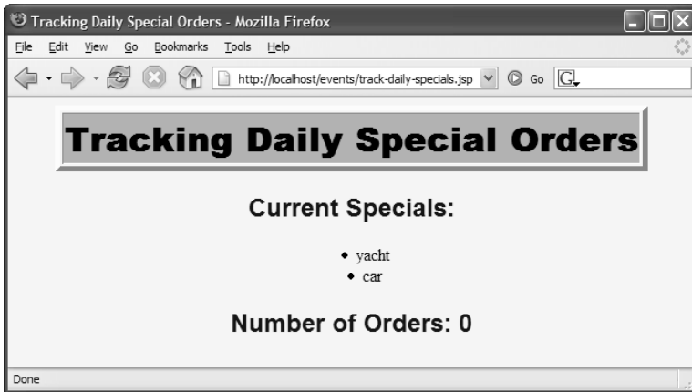
Figure 6–27 When the daily specials are changed, the servlet context attribute listener (Listing 6.41) resets the order count.
