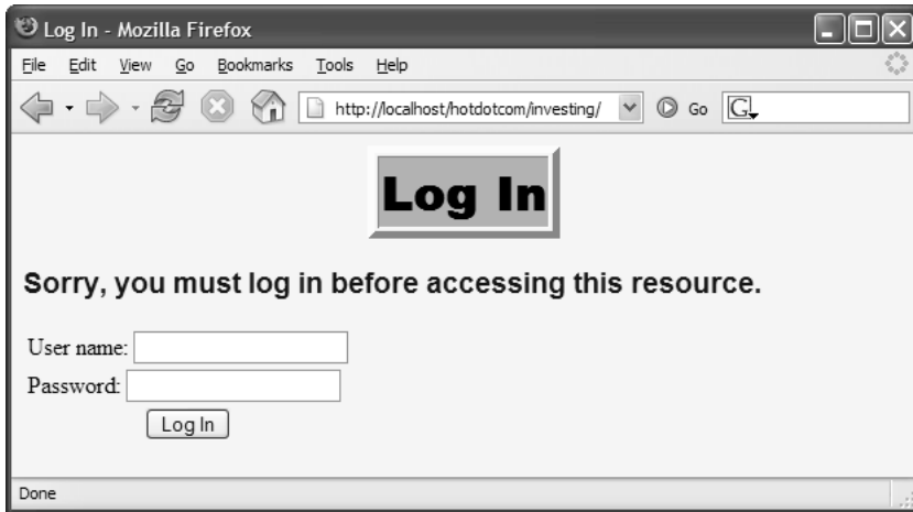
Figure 3–3 Users who are not yet authenticated get redirected to the login page when they attempt to access the investing page.
