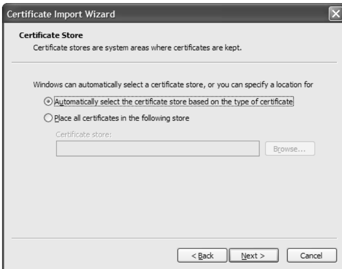
Figure 3–26 Second screen of the Certificate Import Wizard in Internet Explorer. You can let Internet Explorer place the certificate in its default certificate store or choose your own.
