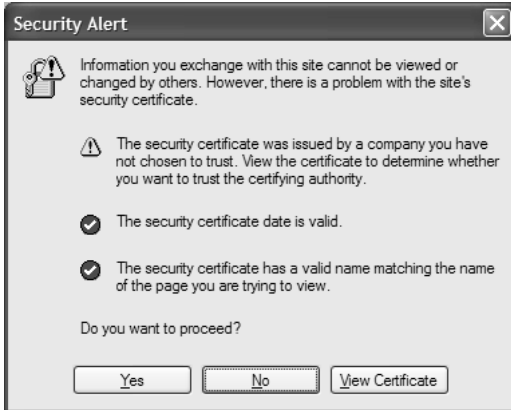
Figure 3–23 Certificate warning dialog box supplied by Internet Explorer. You can view the certificate information by clicking View Certificate.
