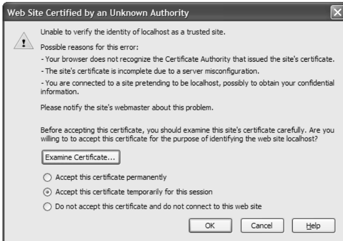
Figure 4–6 New certificate page for Firefox. Examine and accept the certificate permanently to suppress future warnings. For details on creating self-signed certificates for use with Tomcat, see Section 3.7 (Signing a Server Certificate). Again, self-signed certificates would not be trusted in real-world applications; they are for testing purposes only.
