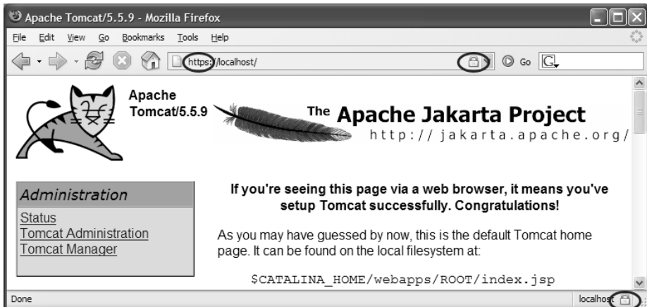
Figure 3–22 After the certificate has been accepted, accessing Tomcat's home page with HTTPS does not produce any warnings (Firefox shown).
