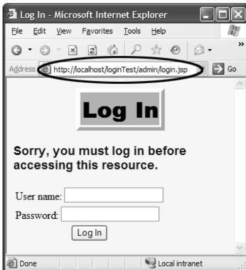
Figure 3–1 When the client tries to access a protected resource, Weblogic 8.1 uses the response.sendRedirect method to send the client to the login page, exposing the login page’s URL.
