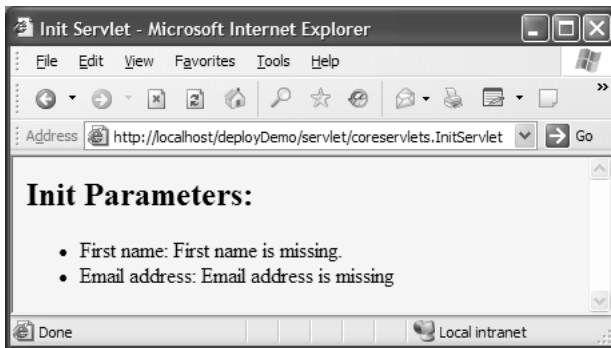
Figure 2-13 The InitServlet when incorrectly accessed with the default URL. Disable the invoker servlet to avoid this problem.
