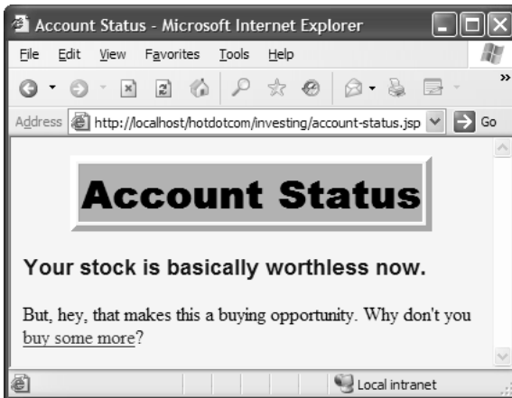
Figure 3–6 Selecting the Account Status link on the investing home page does not result in reauthentication, even if the user has accessed other pages since being authenticated. The system uses a variation of session tracking to remember which users have already been authenticated.
