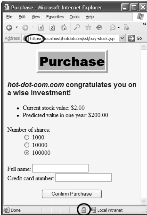
Figure 3-8 The stock purchase page must be accessed with SSL. Because the form's ACTION uses a simple relative URL, the initial form submission uses the same protocol as the request for the form itself.
