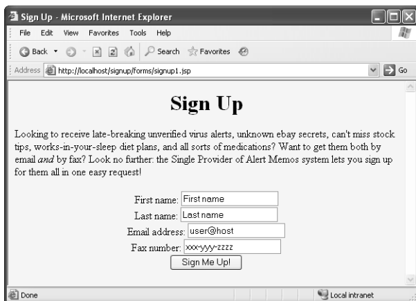
Figure 10–19 Initial registration page. The initial values for the fields are derived from a form bean.
