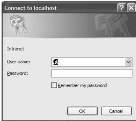
Figure 3–15 Unauthenticated users who attempt to access protected resources are presented with a dialog box. If the authentication fails, the same dialog box will be redisplayed to the user up to three times.
