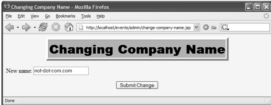
Figure 6-5 The form to change the company name when the page is accessed by an authenticated user who is in the ceo role.
