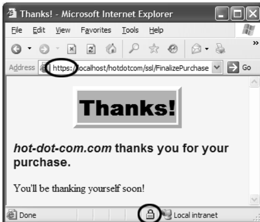
Figure 3-9 To protect the credit card number in transit, you must use SSL to access the FinalizePurchase servlet. Although FinalizePurchaseServlet dispatches to sucker.jsp , no web.xml entry is needed for that JSP page. Access restrictions apply to the client's URL, not to the behind-the-scenes file locations.
