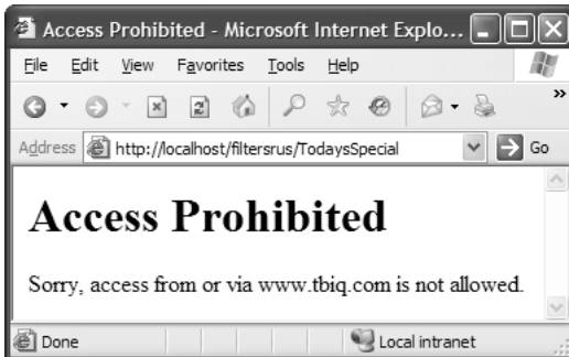
Figure 5-6 You cannot successfully follow the link from the page of Figure 5-5. The BannedAccessFilter prohibits access from www.tbiq.com (an unscrupulous competitor to filtersRus.com ).
