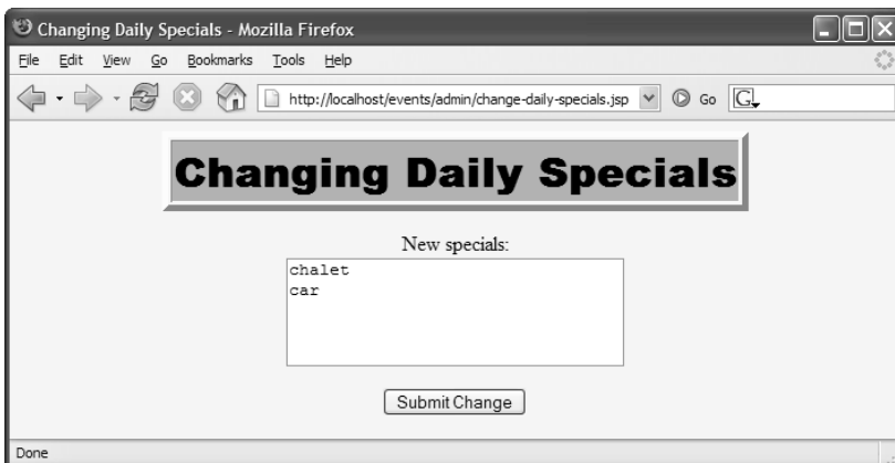
Figure 6–25 Users who pass authentication and are in the designated role ( ceo ) are shown the form for changing the daily specials (Listing 6.42). The current daily specials are displayed as the initial value of the text area.
