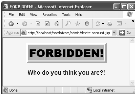
Figure 3–10 When John and Jane attempt to access the Delete Account page, they are denied (even though they are authenticated). That’s because they belong to the registered-user role and the web.xml file stipulates that only users in the administrator role should be able to access this page.
