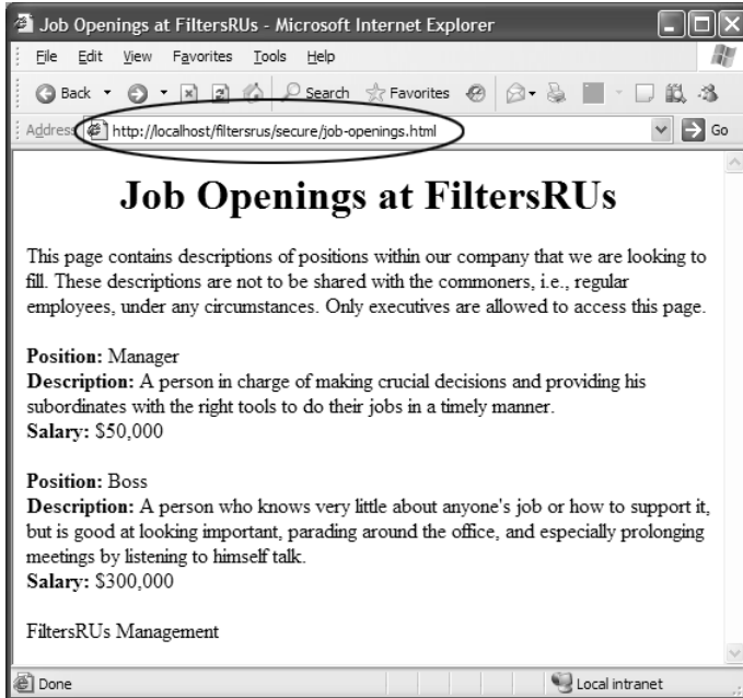
Figure 5-12 Even though the originally requested URL was http://localhost/filtersrus/SecurityHole , the filter forced the client to directly request the resource, thus changing the requested URL to http://localhost/filtersrus/secure/job-openings.html . This screen is shown if the user successfully logs in with a username belonging to the executive role.
