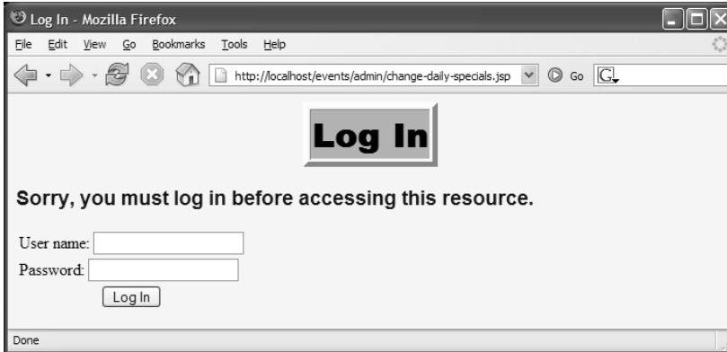
Figure 6–23 Requests by unauthenticated users for change-daily-specials.jsp get sent to the login page (Listing 6.9).
