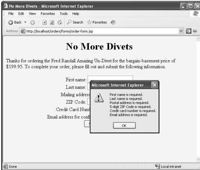
Figure 12–12 Results of submitting the order form with missing fields. Client-side JavaScript validation checks the fields against validation rules and displays a warning dialog box to the user.
