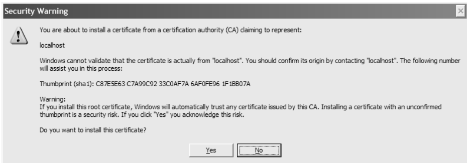
Figure 3–28 Warning dialog box in Internet Explorer making sure you understand that once the certificate is imported, Windows will no longer pop up a warning dialog box, automatically trusting this certificate.
