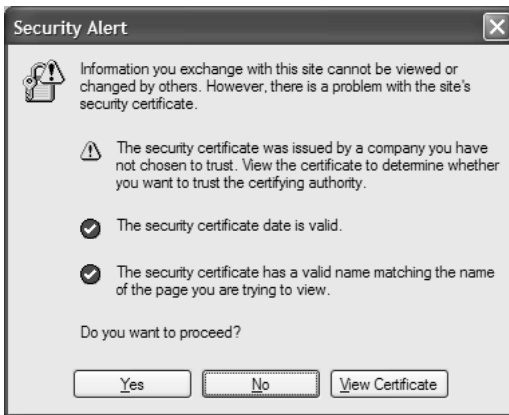
Figure 3-7 Warning when user first accesses FinalizePurchaseServlet when Tomcat is using a self-signed certificate. Self-signed certificates result in warnings and are for test purposes only. See Section 3.5 (Configuring Tomcat to Use SSL) for details on creating them for use with Tomcat and for information on suppressing warnings for future requests.
