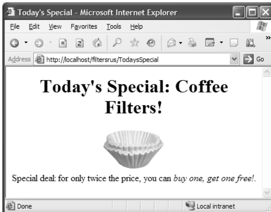
Figure 5–2 Page advertising a special sale. After the page is deployed on an external server and the reporting filter is attached, each client access results in a printout akin to “admin.microsoft.com tried to access http://www.filtersrus.com/filters/TodaysSpecial on Fri Oct 27 13:21:56 EDT 2006.”
