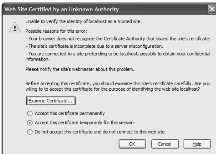
Figure 3–20 Certificate warning dialog box supplied by Firefox. You can view the certificate information by clicking Examine Certificate.
