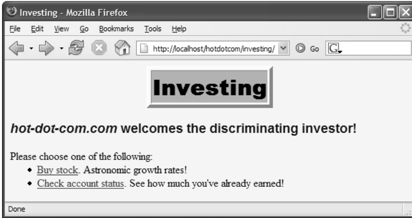
Figure 3–5 Successful login attempts result in redirection back to the originally requested page.
